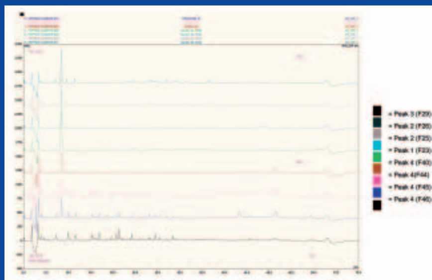
Figure 2. Separation of tryptically digested lysostaphin isoforms on an Acclaim PepMap 300 (C18 3µM 100Å) column using an Ultimate 3000 LC system (Dionex, UK). Separation achieved using a 0-5% B (90% acetonitrile, 0.09% TFA) gradient over 60 min at a flow rate of 100µl/min.
